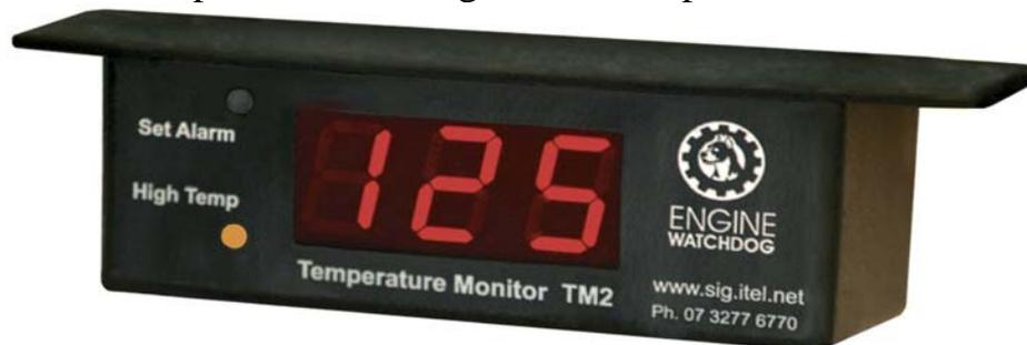
**PRO's...** Constant and accurate readout updated every 2 sec's....very simple to fit. Settable high temperature alarm with audible/visual alarm.
